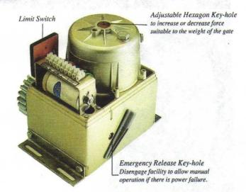
Electromechanical Motor unit consists of small, rugged single block casting containing the worm gear and motor unit. The geared motor unit is of Oil Bath type with Low Component Wear and Excellent Heat Dispersal to ensure maximum reliability.
