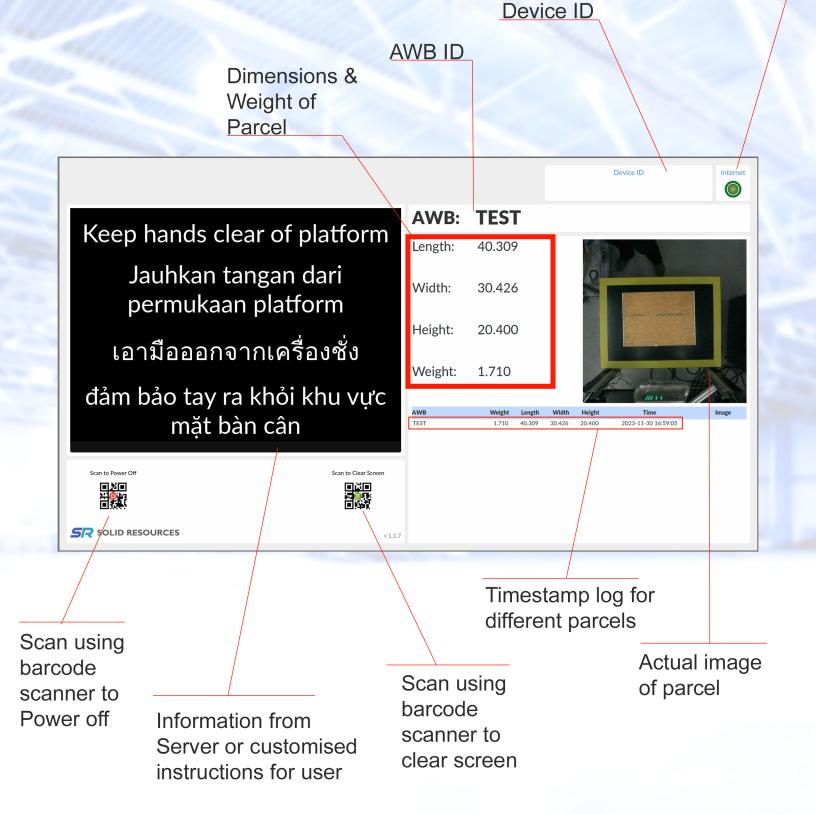
Log files with photos of parcels will be saved and user can extract using usb thumbdrive or through network
